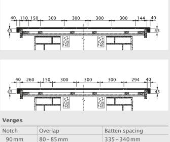
installed in a half offset pattern, whole and half tiles are available. All verge tiles are available with 90 mm and 120 mm notches. You can find information about the relationship of notch to batten spacing in the table.
